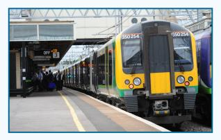
EMU – Electric Multiple Unit. Standard 'heavy rail' Electric Commuter Trains in widespread use across the UK and likely to be rolled out on some/all of the valley lines network following electrification by 2020.
