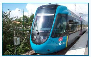
Tram-train: A hybrid train used in parts of Europe, able to run on normal electrified rail lines and also in 'tram' mode on street enabling lower cost extension of rail services. Could work well in Cardiff to link City and Coryton lines to Cardiff Bay and beyond, as well as potential extension to the North West of Cardiff and RCT. The best known example is Karlsruhe in Germany. Currently being trialled in Sheffield.
